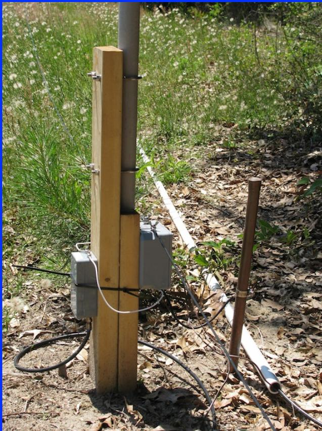
Loop Support, Direction Control Box, Hi-Z Amplifier
