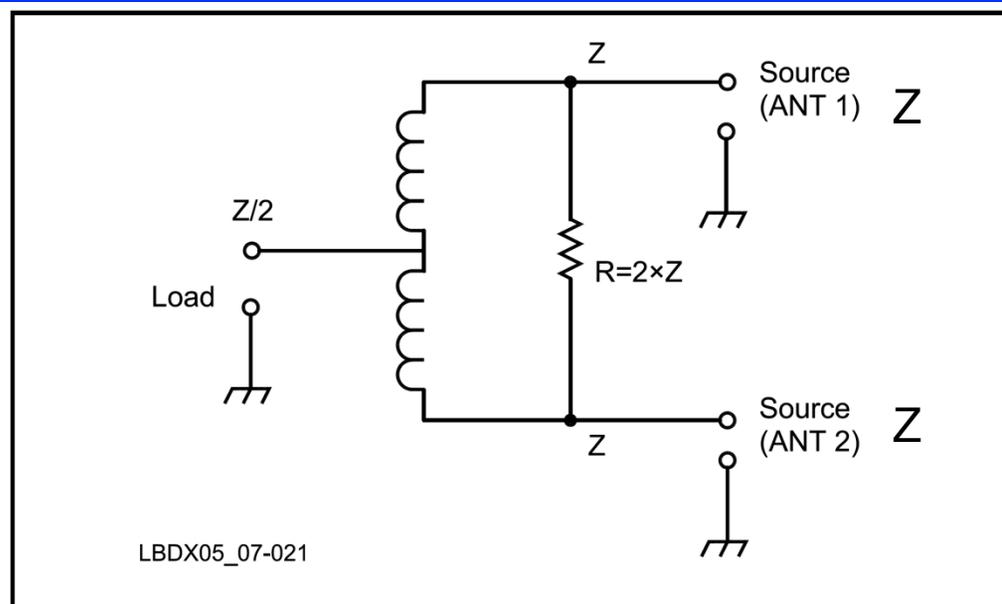
**Fig 7-21 — Simplified schematic diagram of the 0° hybrid combiner.**
